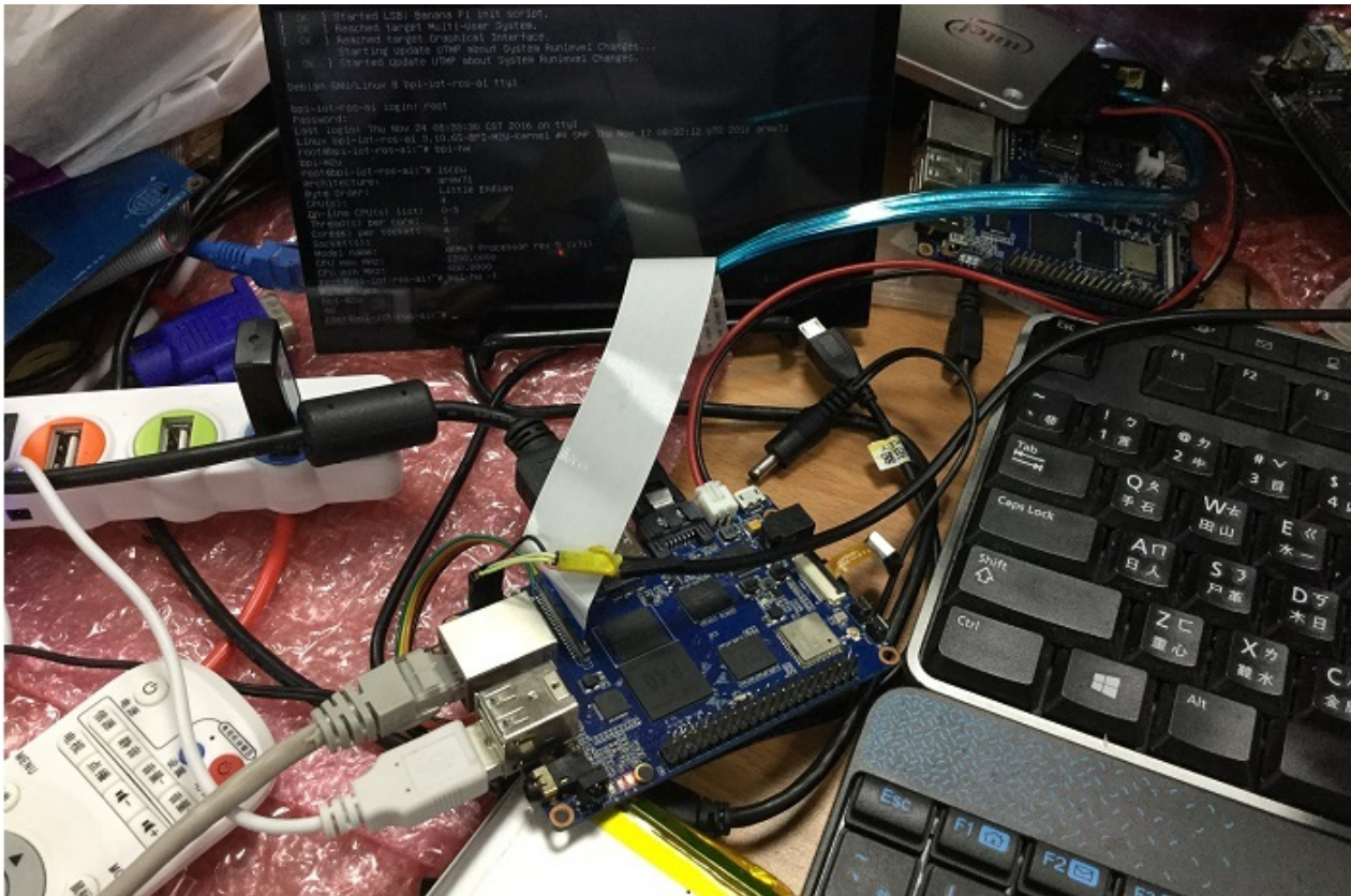
debian 8 with LCD scree and power with lithium battery
