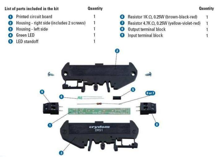
(E) Use 1K Ω (brown-black-red) resistor for applications with control voltage range between 3-15 Vdc and 4.7K Ω (yellow-violet-red) resistor for applications with control voltage range between 15-32 Vdc. LED status indicator is not required for proper function of the SSR and may be omitted. No resistors are needed when LED is not installed. For AC input SSR control applications LED status indicator and resistor must not be used. SSR(s) purchased separately.
