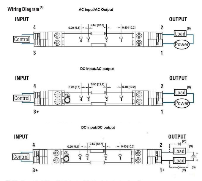
(A) Wiring diagram is identical for each individual section whether it is a single or four channel assembly.
