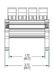
Tolerances: ± 0.02 in / 0.5 m All dimensions are in: inches [millimeters]
