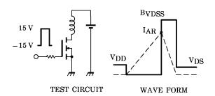
$$\begin{array}{ll} R_G = 25~\Omega \\ V_{DD} = 25~V,~L = 221~mH \end{array} \quad E_{AS} = \frac{1}{2} \cdot L~\cdot I^2 \cdot (~\frac{B_{VDSS}}{B_{VDSS} - V_{DD}}) \end{array}$$
