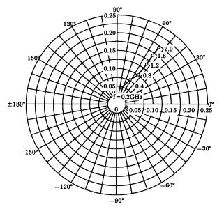
$\begin{array}{l} \text{S}_{22e} \\ \text{V}_{\text{CE}} = 6\text{V} \\ \text{I}_{\text{C}} = 3\text{mA} \\ \text{Ta} = 25^{\circ}\text{C} \\ \text{(UNIT}: \Omega) \end{array}$ j50 j25 j100 j150 j10 j250 10 250 f=0.2GHz-j250 -j10 . -j150 -j100 -j50
