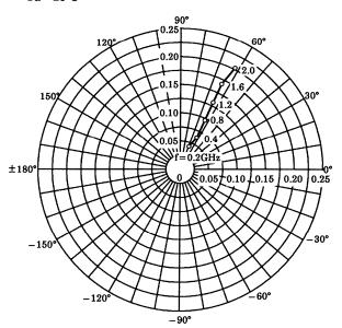
$S_{22e}$   $V_{CE} = 6V$   $I_{C} = 7mA$   $T_{a} = 25^{\circ}C$   $(UNIT : \Omega)$
