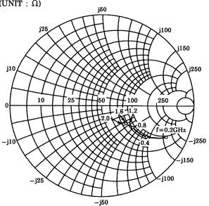
$\begin{array}{l} S_{11e} \\ V_{CE} = 6V \\ I_{C} = 7mA \\ Ta = 25^{\circ}C \\ (UNIT:\Omega) \end{array}$
