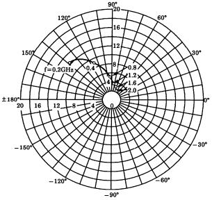
$\begin{array}{l} S_{12e} \\ V_{CE} = 6V \\ I_{C} = 3mA \\ T_{a} = 25^{\circ}C \end{array}$
