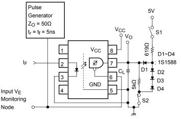
$C_L$  is approximately 15pF which includes probe and stray wiring capacitance.
