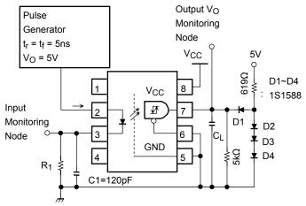
$C_1$  is peaking capacitor. The probe and jig capacitances are include in  $C_1.$   $C_L$  is approximately 15pF which includes probe and stray wiring capacitance.
