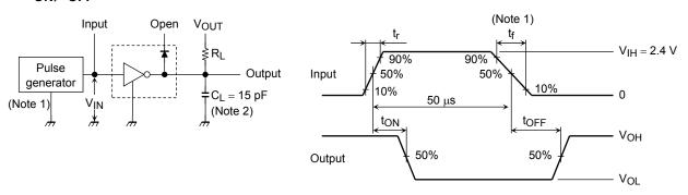
Note 1: Pulse Width 50 μs, Duty Cycle 10%
