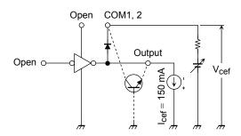
$I_{cef} = 150 \text{ mA} \text{ (at. single pulse} = 5 \text{ ms)}$
