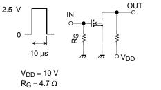
$\begin{array}{l} D.U. \leqq 1\% \\ V_{IN} : t_r, \, t_f < 5 \; ns \\ Common \; Source \\ Ta = 25^{\circ}C \end{array}$
