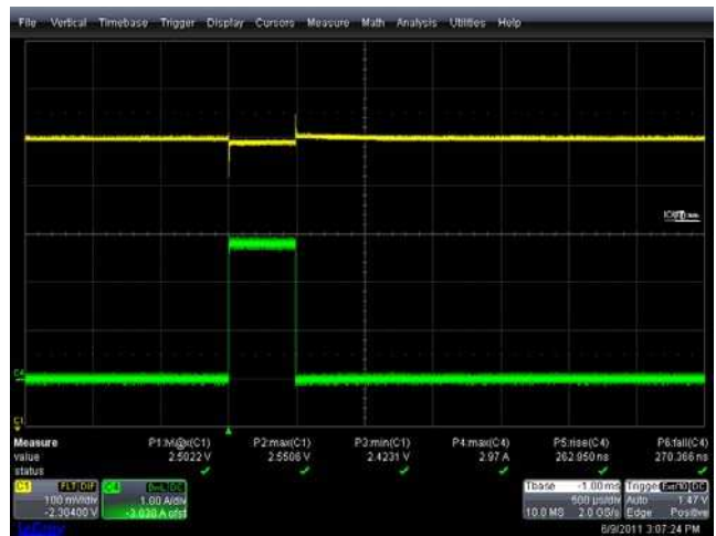
FIGURE 20. TRANSIENT LOAD RESPONSE, V IN = 3.3V, V OUT = 2.5V, C OUT = 220µF, 25mΩ
