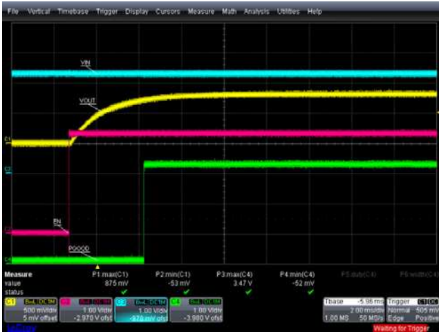
FIGURE 21. POWER-ON AND POWER-OFF, EN = 0 TO 1, +25°C, V_{IN} = 6V , V_{OUT} = 0.8V , I_{OUT} = 0.5A , PGOOD TURN-ON
