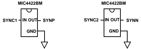
FIGURE 22B. NON-INVERTING DRIVERS
