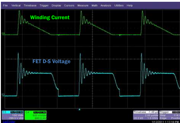
FIGURE 14. QUASI-RESONANT NEAR-ZVS SWITCHING
