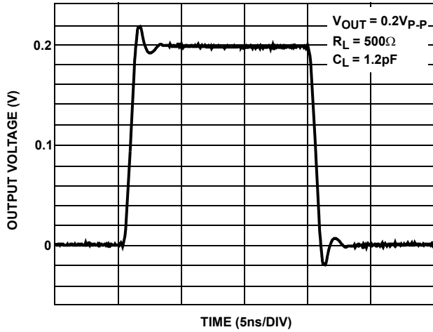
FIGURE 14. SMALL SIGNAL TRANSIENT RESPONSE; R_L = 500\Omega
