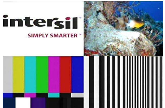
FIGURE 30. TEST PATTERN IMAGE AFTER 3000 FEET OF RG-59 COAX WITH ISL59602 (OR BETTER)
