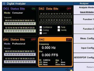
Figure 3: View up to four channels - two for analog, two for digital - at the same time for multiple analyses.
