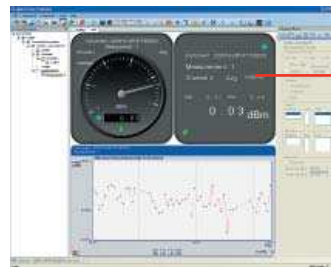
Multiple channel list and measurement math
