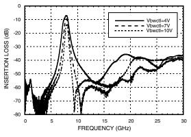
Insertion Loss vs. Vbwctl, Vfctl = 7V
