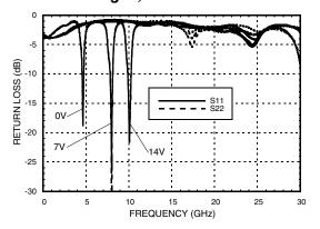
Return Loss vs. Control Voltages, Vfctl = Vbwctl
