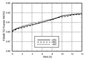
Tuning Sensitivity vs. Temperature, Vfctl = Vbwctl
