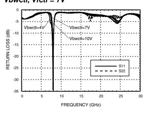
Return Loss vs. Vbwctl, Vfctl = 7V
