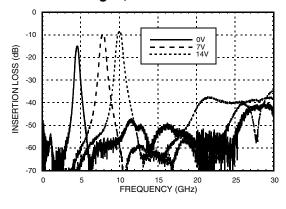
Insertion Loss vs. Control Voltages, Vfctl = Vbwctl
