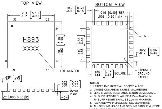
SOLDERED TO PCB RF GROUND. 7. REFER TO HITTITE APPLICATION NOTE FOR SUGGESTED LAND PATTERN.
