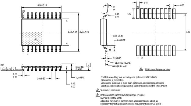
All pads a minimum to U20 mini rom an adjacent pads, adjast as necessary to meet application process requirements and PCB layout tolerances; when mounting on a multilayer PCB, thermal vias at the exposed thermal pad land can improve thermal dissipation (reference EIA/JEDEC Standard JESD51-5)
