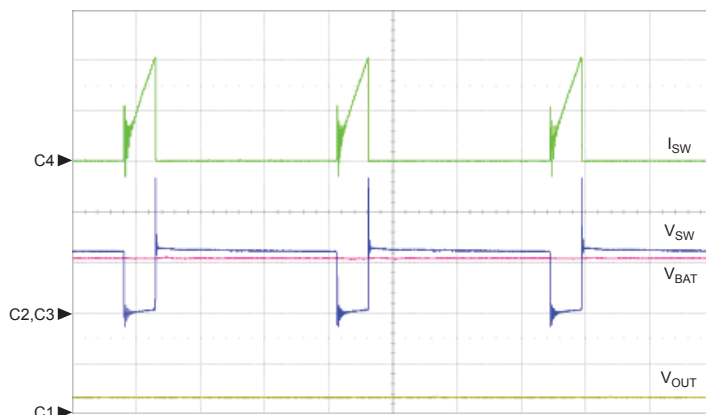
Figure 3. Expanded view of Timer mode: V_{OUT} \leq 10 V, V_{BAT} = 5.5 V, Ch1: V_{OUT} = 20 V/div., Ch2: V_{BAT} = 5 V/div., Ch3: V_{SW} = 5 V/div., Ch4: I_{SW} = 500 mA/div., t = 5 \mu s/div.
