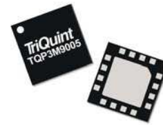
16-pin 3x3 QFN package
