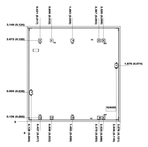
Units: millimeters (inches) Thickness: 0.100 (0.004) (reference only) Chip edge to bond pad dimensions are shown to center of bond pad Chip size tolerance: +/- 0.051 (0.002)
