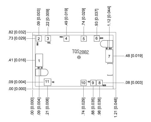
Units: millimeters [inches] Thickness: 0.10 [0.004] (reference only) Chip edge to bond pad dimensions are shown to center of bond pads. Chip size tolerance: ±0.05 [0.002] RF ground through backside
