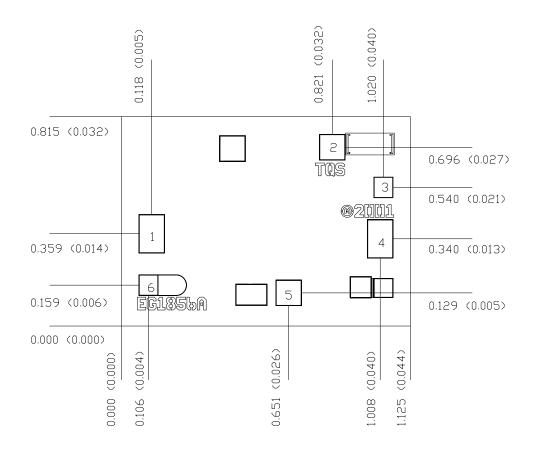
Units: millimeters (inches) Thickness: 0.1016 (0.004)
