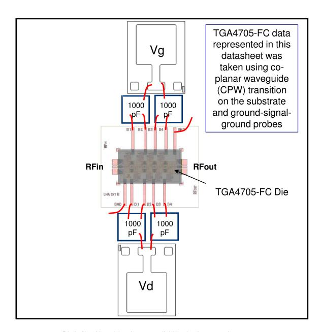
Die is flip-chip soldered to a 15 mil thick alumina test substrate
