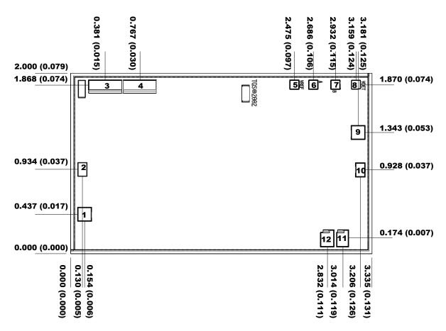
**Units: millimeters (inches)** Thickness: 0.100 (0.004)
