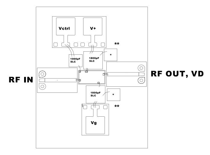
Note: Input and Output ports are DC coupled.
