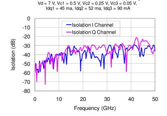
TGA4947-SL Dual Driver Isolation vs Frequency
