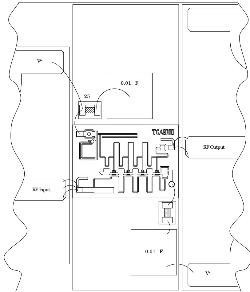
RF connections: Bond using three 1-mil diameter, 20 to 30-mil-length gold bond wires at RF input and two 1-mil diameter, 20 to 30 -mil-length gold bond wires at RF output for optimum RF performance.
