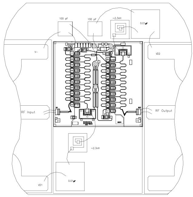
RF connections: Bond using two 1.0-mil diameter, 20 to 30-mil-length gold bond wires at both RF Input and RF Output for optimum RF performance.
