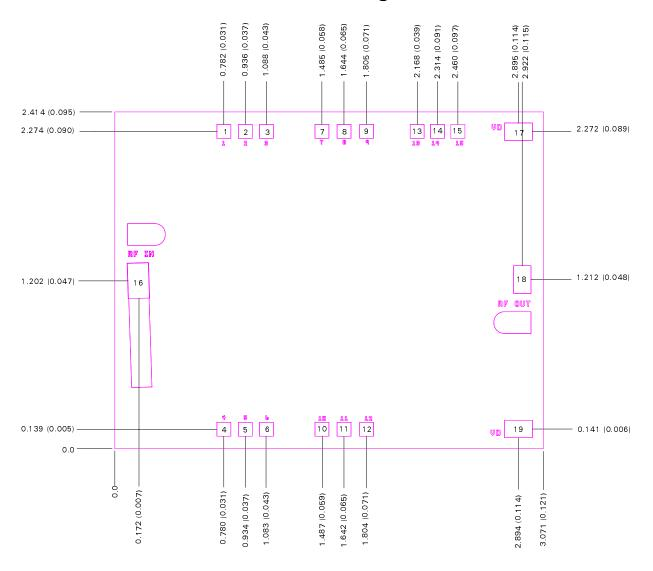
Units: millimeters (inches) Thickness: 0.150 (0.006)
