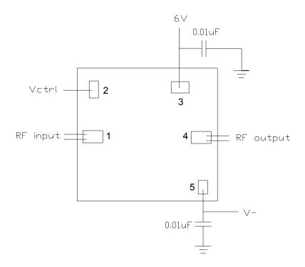
RF connections: Bond using two 1.0-mil diameter, 20-mil-length gold bond wires at both RF Input and RF Output.
