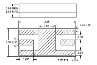
Dimensions shown are nominal in millimeters All tolerances are  $\pm 0.13$ mm except overall length and width  $\pm 0.25$ mm
