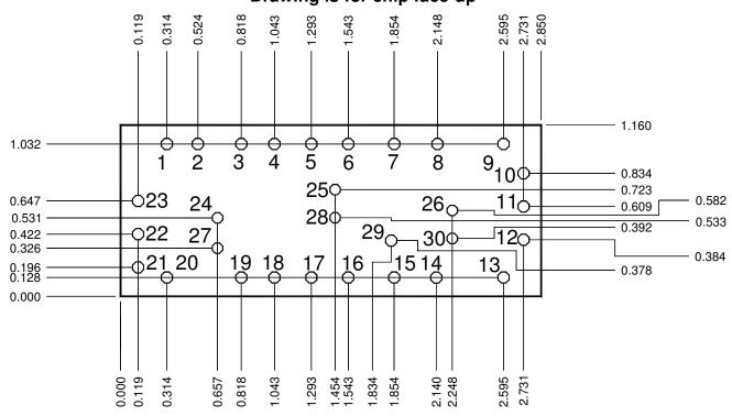
Units: millimeters Thickness: 0.380
