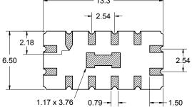
Dimensions shown are nominal in millimeters All tolerances are ±0.15mm except overall length and width ±0.10mm
