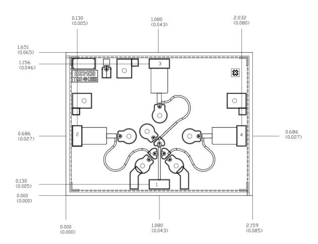
Units: millimeters (inches) Thickness: 0.100 (0.004)
