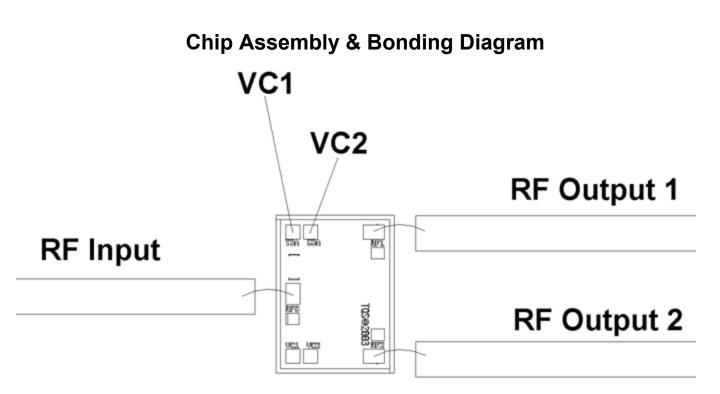
For optimum insertion loss and return loss, a single 0.001" bondwire of length 35 mils should be used. This will be approximately 0.42nH. Differences in bondwire length will have an impact on switch performance.
