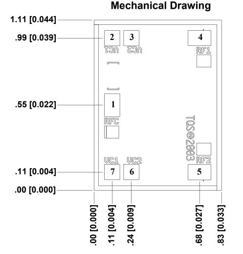
Units: millimeters [inches] Thickness: 0.10 [0.004] (reference only) Chip edge to bond pad dimensions are shown to center of bond pads. Chip size tolerance: ±0.05 [0.002] RF ground through backside
