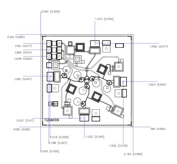
Units: millimeters (inches) Thickness: 0.100 (0.004)
