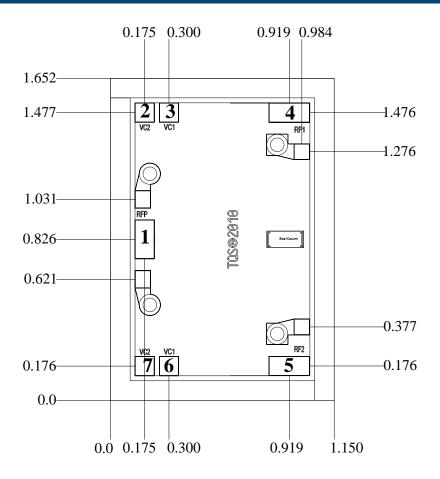
Unit: millimeters Thickness: 0.10
