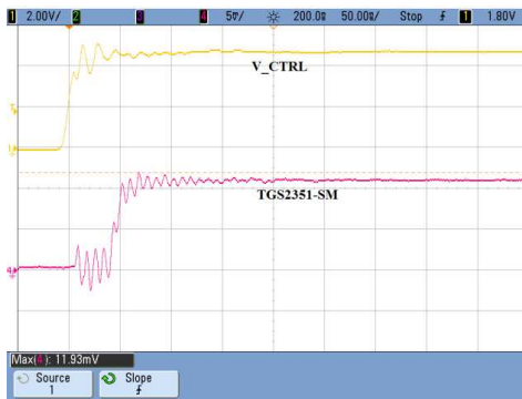
Switching Speed – On 50 ns Vc = 0/-40 V, Freq = 3 GHz, Pin = 30 dBm, +25 °C
