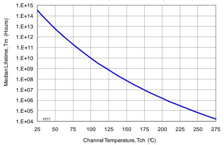
Median Lifetime (Tm) vs. Channel Temperature (Tch)
