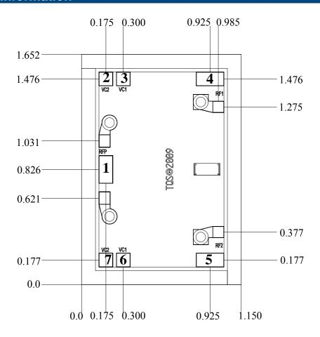
Unit: millimeters Thickness: 0.10
