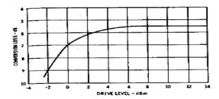
Conversion Loss vs. Drive Level: Conversion loss in an SSB system is a function of drive level (f<sub>1</sub> with f<sub>2</sub> and f<sub>3</sub> at approximately 3 GHz and f<sub>4</sub> level at -6 dBm.
