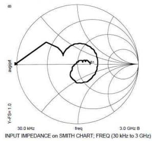
Note: All measurements performed on Hewlett Packard 8753D Network Analyzer (201 sample points, linear scale) in a 50 ohm coplanar waveguide environment. Tables created using MDS software.
