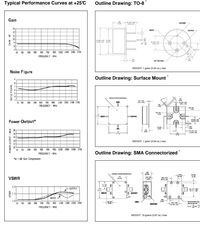
\* Dimensions are inches (millimeters) ±0.015 (0.38) unless otherwise specified.
