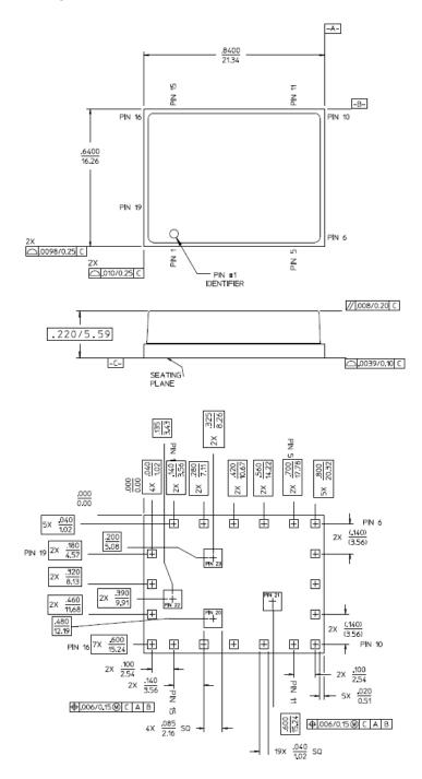
$<sup>^{\</sup>dagger}$  Reference Application Note M538 for lead-free solder reflow recommendations. Meets JEDEC moisture sensitivity level 1 requirements.
