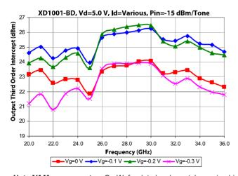
Note [1] Measurements - On-Wafer data has been taken using bias conditions as shown. Measurements are referenced 150 um in from RF In/Out pad edge. For optimum performance M/A-COM Tech T-pad transition is recommended. For additional information see the M/A-COM Tech "T-Pad Transition" application note.
