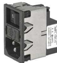
Fig. 15a External filter to reduce conducted emissions of LW models with feature E ( L_1 = L_2 = 1.6\text{ mH} , C_x = 47\text{ nF} , C_y = 2.2\text{ nF} )
