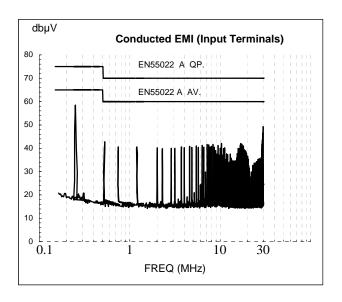
To meet class B for the above standards, it is necessary to fit a 3.3  $\mu\text{F}$  ceramic capacitor across the input terminals.
