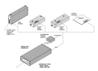
Typical Capacity: Control a subsystem consisting of 32 individual 8-cell programmable attenuators plus 16 DPDT switches.
