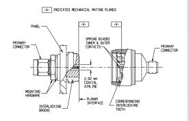
**Axial Isolation of the Center Contact** - Any excessive axial force on the Crown center contact is absorbed by the spring biasing at the Planar interface end.
