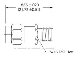
Note: Dimensions in Brackets are Expressed in Millimeters and are for Reference Only. Design specifications are subject to change without notice. Contact factory for technical specifications before purchasing or use.
