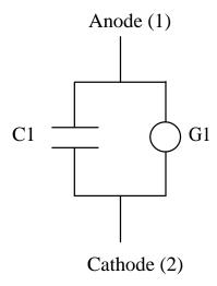
G1 models the reverse and forward bias IV curve. The model does not accurately represent the negative differential resistance region of the IV curve (from the peak to the valley of the IV curve). Also the model does not contain temperature effects. Range for C1 is 0.21 to 0.63pF
